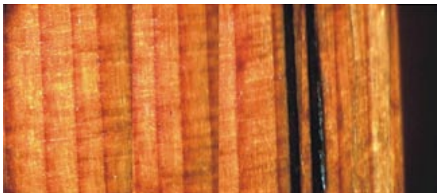
Henri D. Grissino-Mayer had the opportunity to investigate the tree rings on the "Messiah" violin and took this mosaic (photo © H.D. Grissino-Mayer). The wood used by Antonio Stradivari and all Cremonese violin makers for the violin top was Norway spruce ( Picea abies ).
